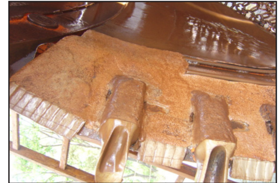
After 20 months only 5 kg of ARC was needed for repair
